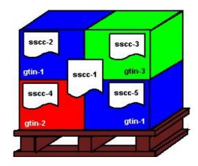
Figure A-1: Heterogeneous content, labels on pallet and cases
