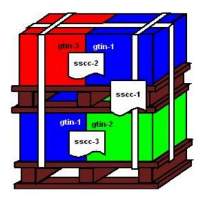
Figure 4-13: Heterogeneous content, sandwich pallet with "master" label
