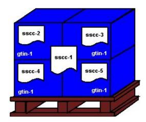
Figure 4-6: Homogeneous content, labels on pallet and cases
