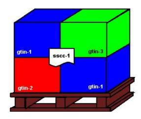
Figure 4-5: Heterogeneous content, label on pallet
