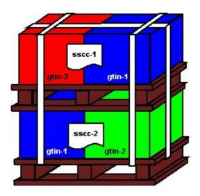
Figure 4-12: Heterogeneous content, sandwich pallet
