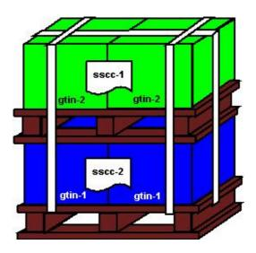
Figure 4-10: Homogeneous content, sandwich pallet
