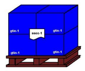
Figure 4-4: Homogeneous content, label on pallet
