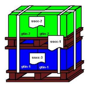
Figure 4-11: Homogeneous content, sandwich pallet, with "master" label
